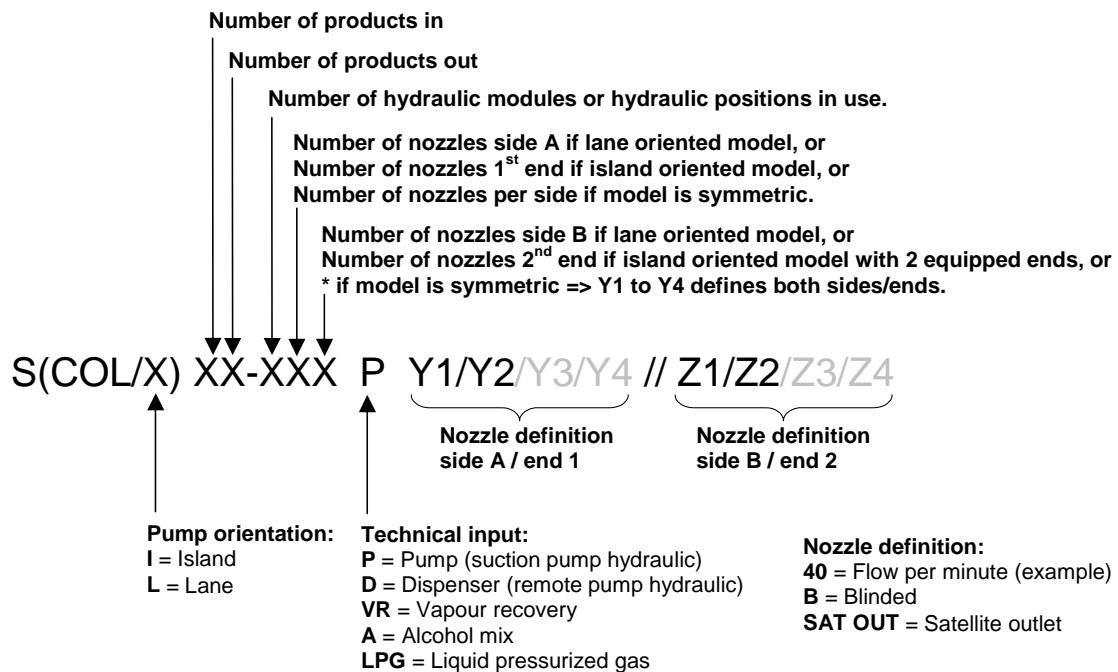
Figure 2 What does the model name of the pump indicate
